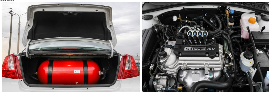
1-rasm. GBU bilan jihozlangan holatda "UzAuto Motors" AJ tomonidan ishlab chiqarilayotgan Lacetti SX CNG L3-15G avtomobili
