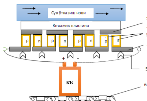
3-rasm. TBlarni kondensator batareyasiga ulanish sxemasi. 1, 4-mos holda, TELarning issiq va sovuq uchlaridagi kommutatsion plastinalar (Fe va Ni), 3-r – va n-tipli termoelementning yarim shoxchalari ( \text{Bi}_2\text{Te}_3 – \text{BiSb}_3 \text{Bi}_2\text{Te}_3 – \text{Bi}_2\text{Se}_3 ), 5-TB ni ko'tarib turish uchun taxta tirkamalar, 6-KB turgan yer sathi
