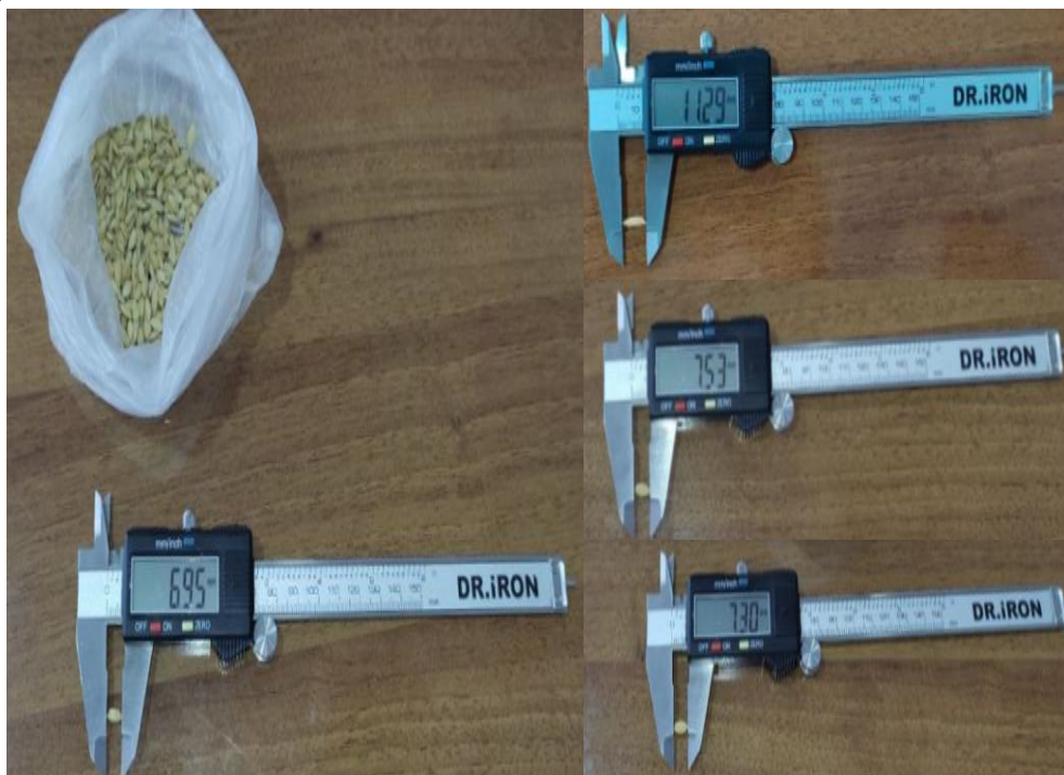
1-rasm. Sholi donini DR.iRON shtangenserkuli bilan o'lchash jarayoni
