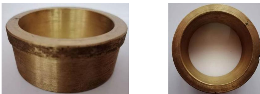
2-rasm. Beshinchi sinf aylanma kinematik juftlikning BrO 8 S 12 markali bronza vtulkasi (tashqi silindr)
